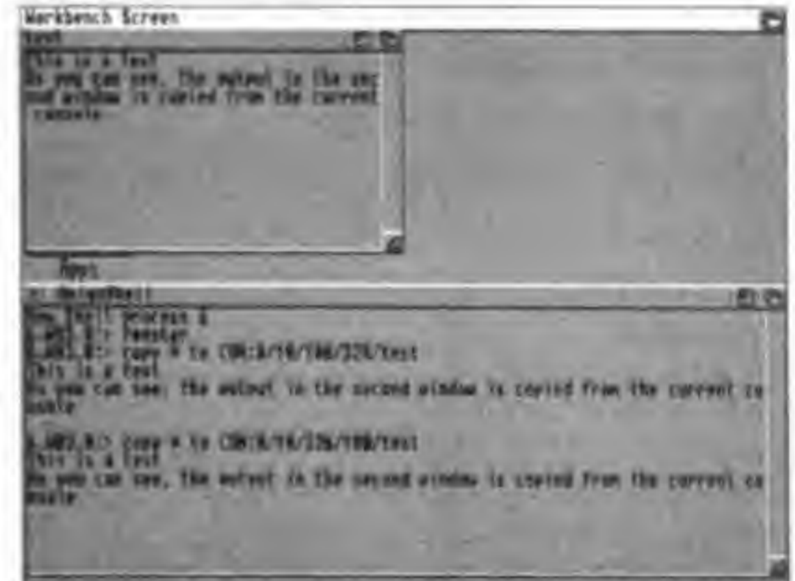
Copying text from the current console to a user-defined file – in this case, in fact, a window.
